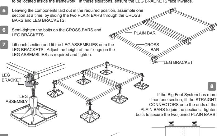
Tighten the entire framework and position condenser units on CROSS BARS.If suitable, use the CLAMPS provided to secure
